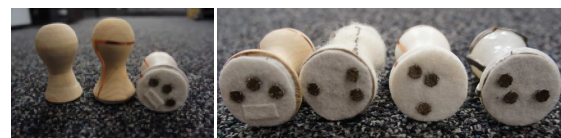
Figure 3. Stampies with a unique conductive pattern
